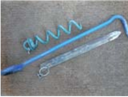
Two kinds of anchor: angle iron stake (below) and corkscrew (above). The man-hole cover lifter (centre) makes an excellent extraction tool for both anchors.
