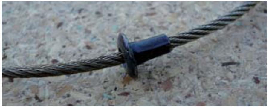
One kind of fixed stop, which prevents the noose closing too far.
