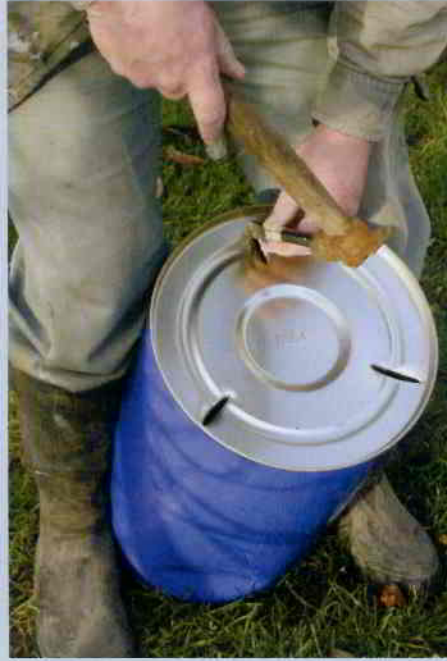
STEP 2. Cut slots in the base with a hammer and cold chisel. These can be adjusted for food flow. Open with twist of a screwdriver, close by tapping from inside with a hammer.
