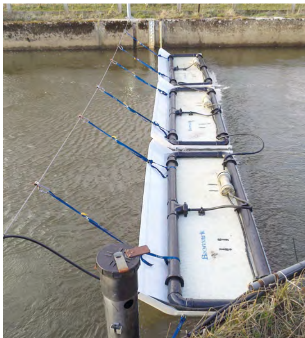
Floating PIT-tag antennae are part of the PIT-tag systems on the River Frome at East Stoke.
