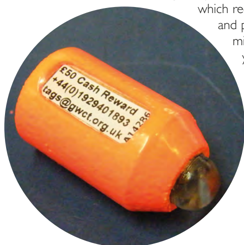
Figure 1 The Data Storage Tag is inserted in an orange float to make it buoyant
