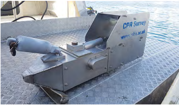
The Continuous Plankton Recorder sampler which samples levels of zooplankton. © Marine Biological Association
