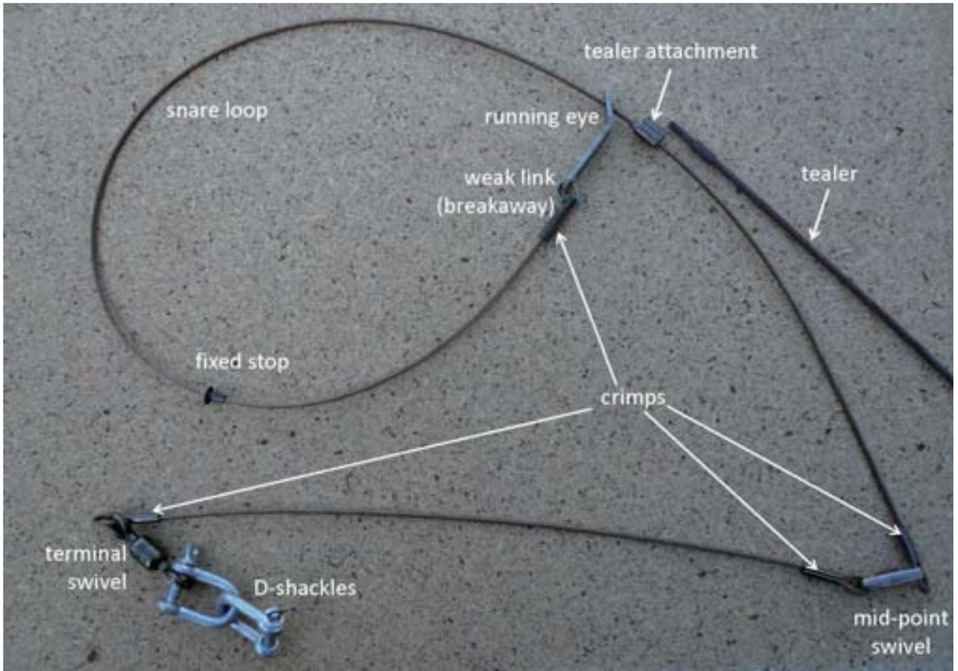
Because snares are such minimalist devices, crucial features are very small details with inter-related functions. Here we describe each component in turn.
