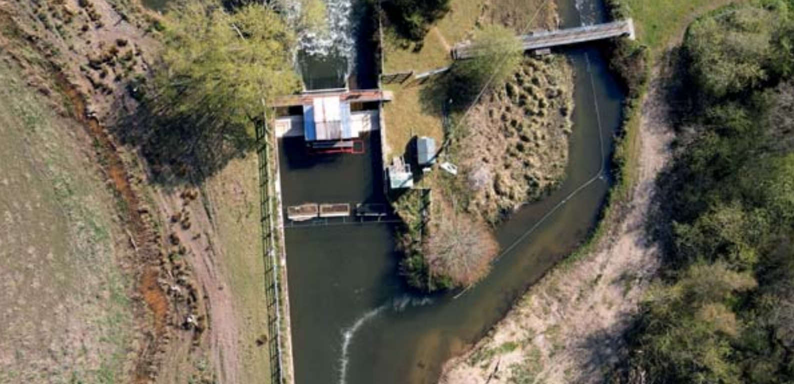
Aerial image of the Bio-Acoustic Fish Fence diverting the smolts down the Millstream immediately upstream of the floating PIT-tag antennae and fish counter on the main river.
