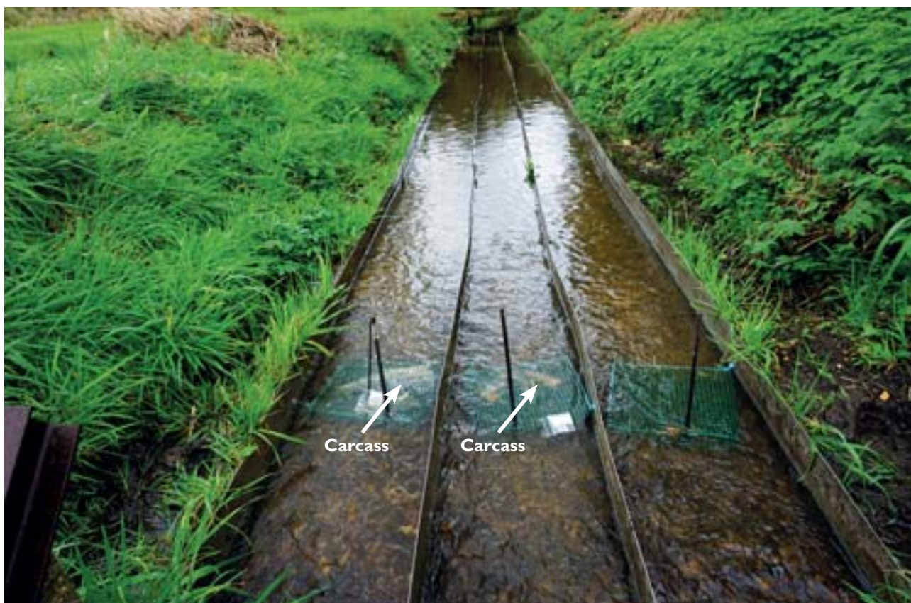
Figure 1 One of four sets of three experimental channels at East Stoke used to study the impact of pink salmon carcasses
