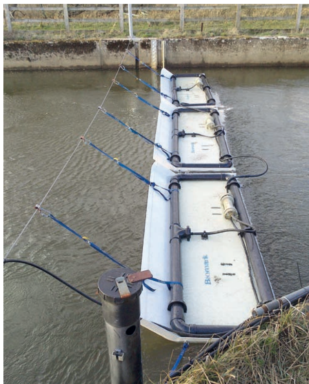
Figure 17 Floating PIT-tag antennae are part of the PIT-tag systems on the River Frome at East Stoke
