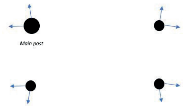
Figure 3: Showing direction tension should be set on corner posts using rope and corner pegs
