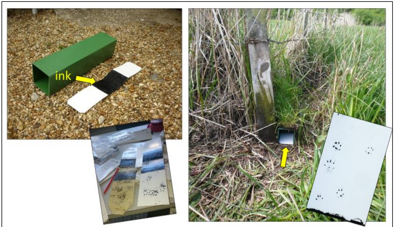
Tunnels made from square-section plastic were set in suitable locations and fitted with an inked card to record small predator footprints.
