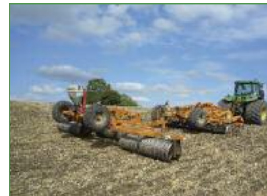
Many local crops are established without ploughing. A Cultipress with Cambridge roller at Loddington. © Alex Butler
