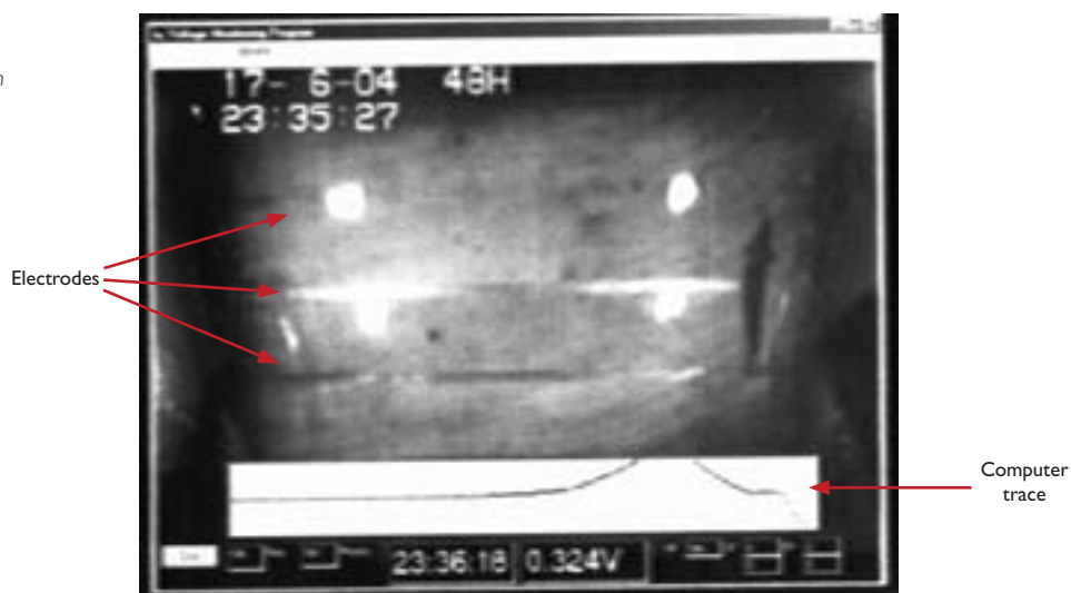
Screen display from the computerised counting and evaluation system. The image shows a 75cm salmon ascending the weir
