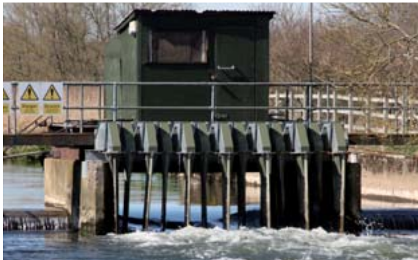
PIT tag data is collected by detection vanes mounted on the main river counter.
