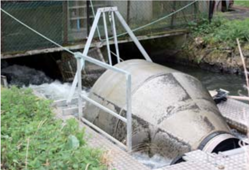
There are concerns that Rotary Screw Traps, used to trap and count migrating salmon smolts on rivers, may be detrimental to the fish.
