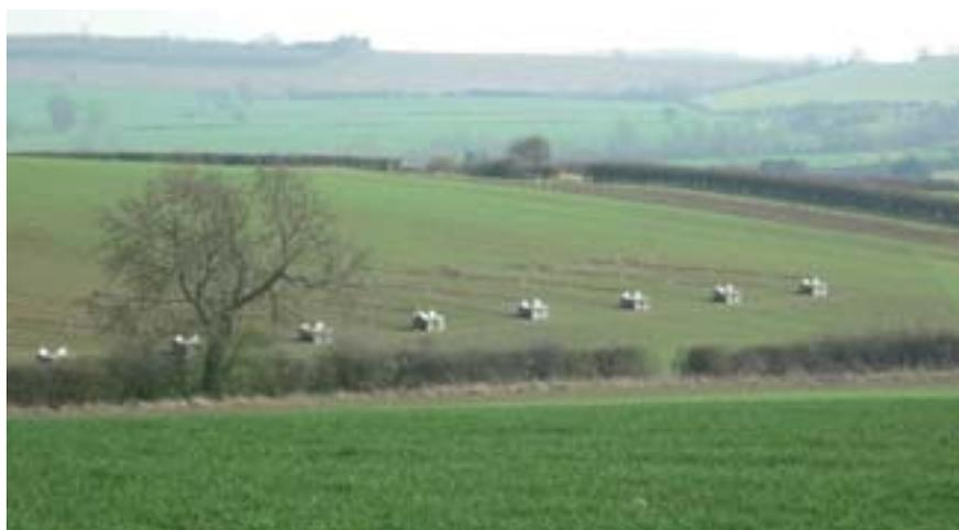
*Run-off from the tramlines was collected in these tanks and measured.* © Alastair Leake/GWCT
