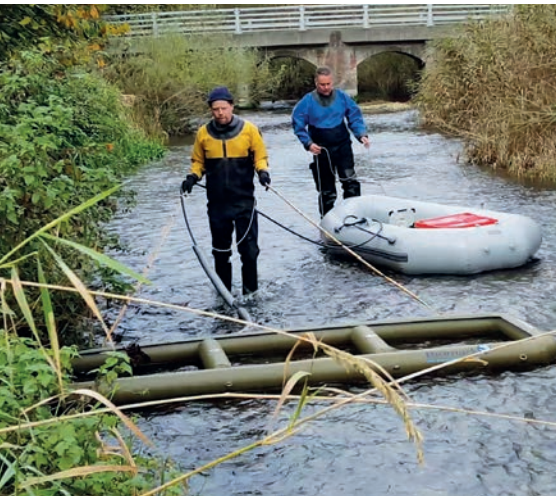
Wading downstream with the inflatable PIT tag antenna (green device) which links to a GPS enabling us to determine the distance travelled by individual fish during the autumn shift.
