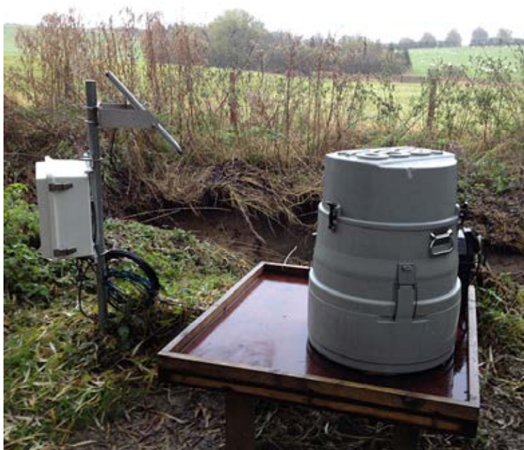
Figure 13. Automated water sampling equipment is installed at the downstream end of each stream catchment. We are using this equipment to near-continuously monitor nutrient and sediment concentrations. In the autumn when surface runoff and drainflow normally restarts, we are using this equipment to samples for pesticides. The photograph shows an Isco sampler on the right with a solar powered data logger .
