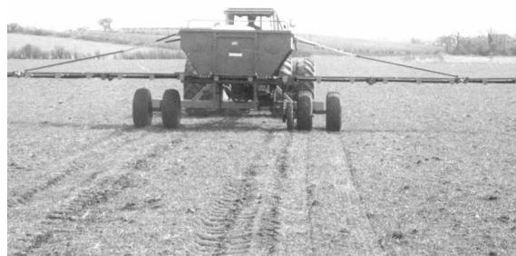
Figure 3 Fitting extra tyres and lowering inflation pressures minimises the risk of subsoil damage (Photo: Silsoe Research Institute)
