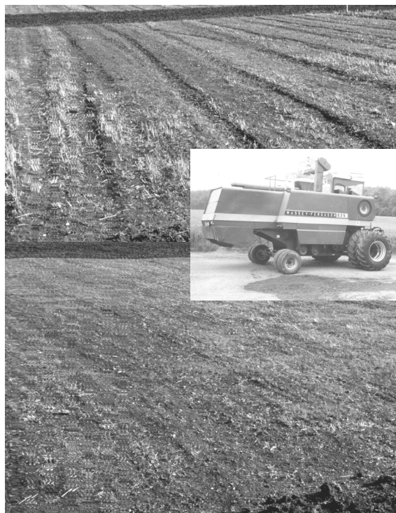
Figure 4 These plots were harvested on the same day by the same machine but with single wheels (top) and with dual wheels (inset) at lowered inflation pressure (bottom) (Photos: Silsoe Research Institute)
