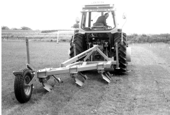
Figure 2 Slant leg subsoiler working in grassland. This machine can provide good fissuring without extensive disruption and loosening
