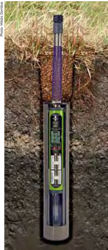
Probes buried in the soil capture and count the microfauna
