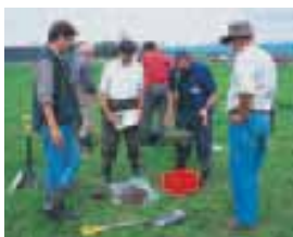
Photo 2.9 The drop shatter test in action. The sample is dropped a maximum of 3 times from a height of 1 m (waist height) onto the wooden square in the plastic basin. The soil is then transferred onto the large plastic bag and graded so that the coarsest clods are at one end and the finest aggregates are at the other end.
