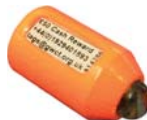
(Above) An acoustic transmitter which emits a ping every 30 seconds that will be picked up by the receivers. (Below) The data storage tag will be inserted into the fish and will record temperature and depth every two minutes.
