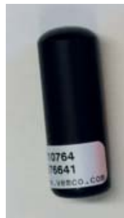
(Above) An acoustic transmitter which emits a ping every 30 seconds that will be picked up by the receivers. (Below) The data storage tag will be inserted into the fish and will record temperature and depth every two minutes.
