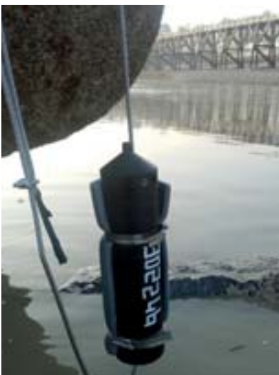
The acoustic receivers are programmed and then placed in the lower rivers and estuaries.
