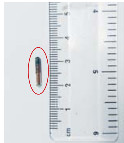
(Above) We electric-fish and tag approximately 10,000 juvenile salmon. (Below) The PIT tags are just 12mm long x 2mm in diameter.
