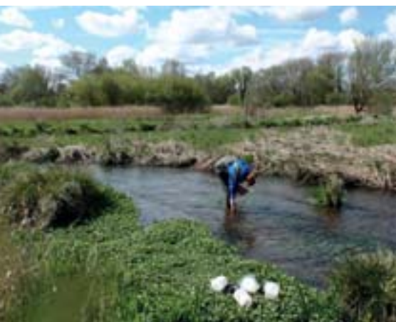
Jessica using a Surber sampler to sample the macroinvertebrate community.
